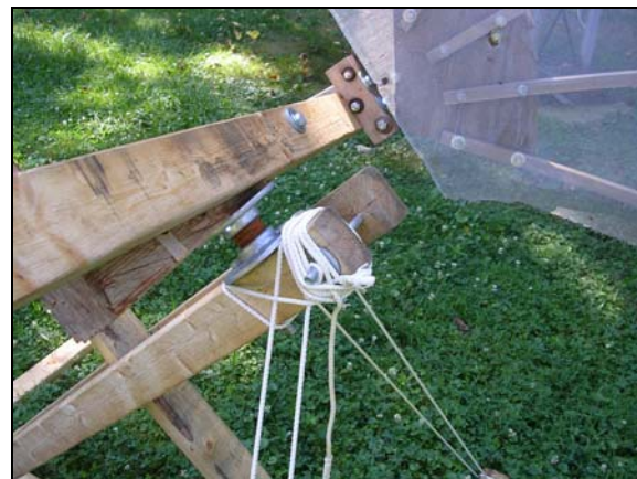
Figure 8. 1" diameter pipe nipple is used for the polar axis
