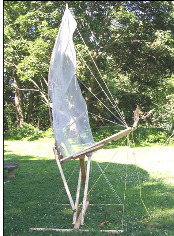
Figure 1. 7.5' offset dish on polar mount
