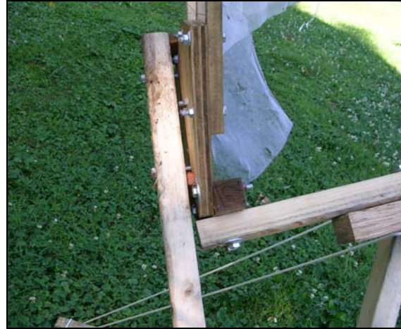
Figure 5. The dish is attached to the feed support by a 2" x 2" block
