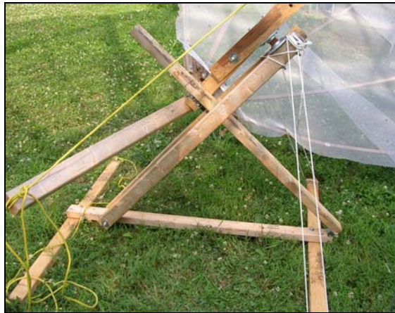
Figure 7. The base of the polar mount is made from six 4' length of 2" x 3" lumber
