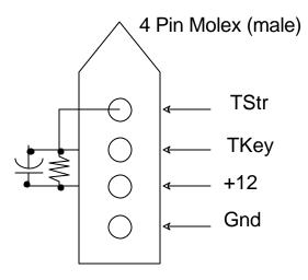
R=10k, C=1000  $\mu$ f This will provide 10 sec cw @ 10 watts when "Tune" button on 706 is pressed
