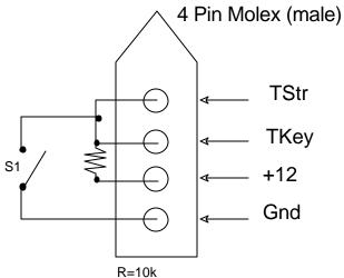
This configuration will provide 3 sec of 10 w cw when "Tune" button is pressed or 10 w cw for as long as S1 is closed. If S1 is replaced with a relay Tune function can be controled by power to a screwdriver antenna
